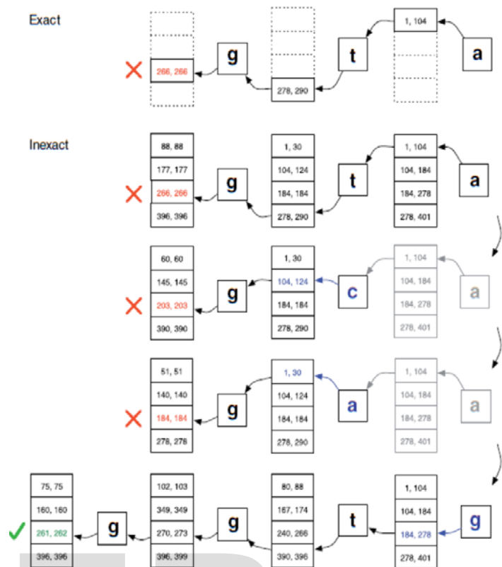
Fig. 6. Example of running the inexact match variant of the Bowtie algorithm. In this example, we try to map the string 'ggta' to the genome, but we only succeed at mapping 'gggtg'. The array at each level of the backtracking shows the row intervals corresponding to suffixes with the 4 nucleotides at that position (in the order a, c, g, t). Source: [1].
